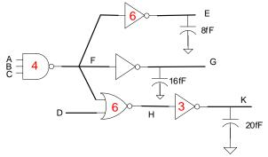
Problem 3A segment of a logic block is shown below. Assume the lengths of<br/>all devices are  $L_{MIN}$ . Assume all gates are sized for equal worst-case rise and fall times.
